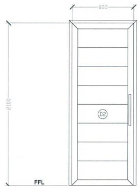
1 SET PANEL DOOR IN 2"X5" TANGUILE / MAHOGANY DOOR JAMB; USE 4 PCS 4" HEAVY DUTY HINGES; & HEAVY DUTY DOOR KNOB
