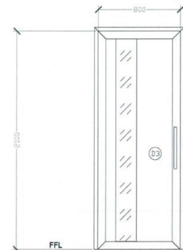
1 SET FLUSH DOOR, DOUBLE WALL WITH 1/2" THK. PLYWOOD WITH INSTALLED CLEAR GLASS IN 2"X5" TANGUILE / MAHOGANY DOOR JAMB; USE 4 PCS 4" HEAVY DUTY HINGES; & HEAVY DUTY DOOR KNOB
